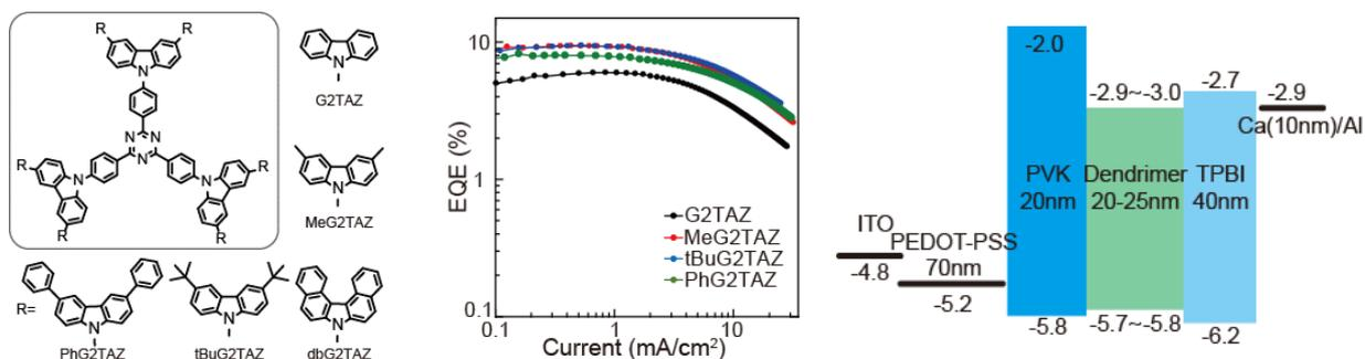
Fig.1 (left) Structure of terminal modified second generation carbazole triazine dendrimers. (middle) External quantum efficiency-current density characteristics for OLEDs with fully solution processed organic layers containing TADF dendrimers as an emitter. (right) Energy diagram of the OLED device.
