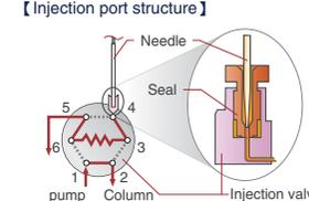
Removal of dead volume through the direct connection between the injection port and the injection valve.
