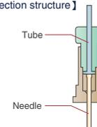
Removal of dead volume from needle Connection by means of a flange needle (without a ferrule).
